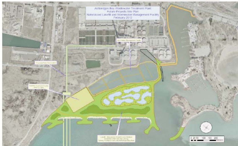
Ashbridges Bay Landform Concept Incorporating Stormwater Management Wetland and Combined Sewer Overflow High Rate Treatment Facility
