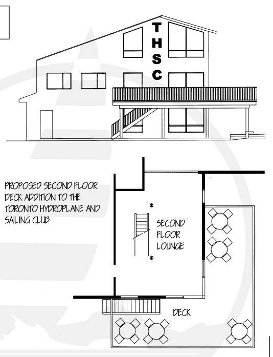
construction meets the load requirements set by the engineers and the Ontario Building code administered by the Building Department. Besides load factors, we have to adhere to safety requirements both during construction and after, meaning deck and stair railings.
